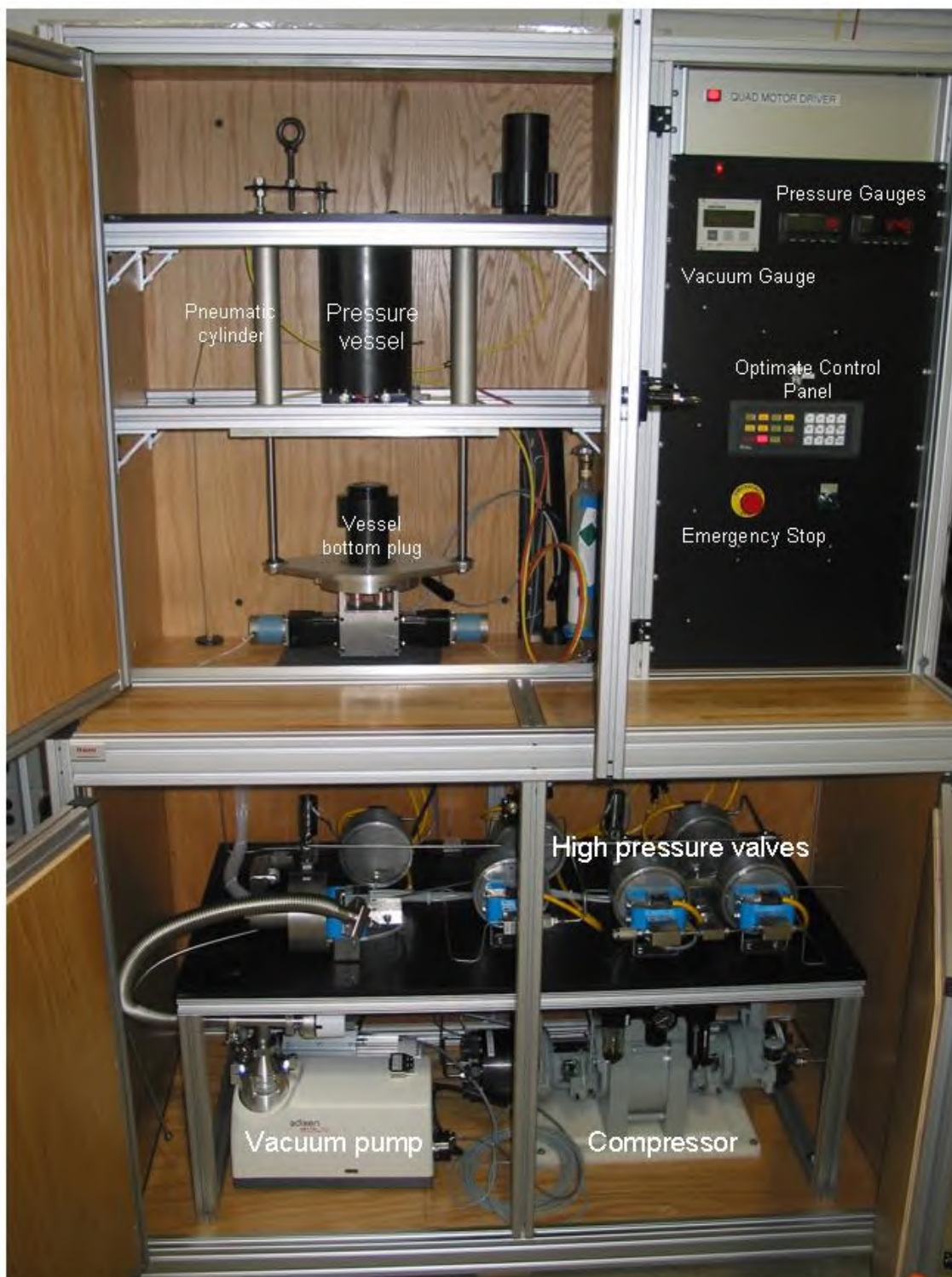
Figure 2. Annotated photograph of gas loading system
