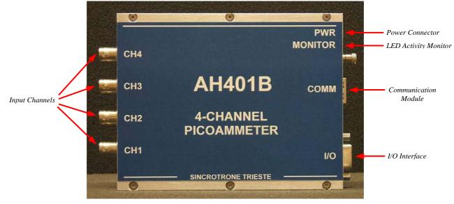
Fig. 1 - The AH401B I/O Connections
