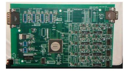
FIG 2C. A photograph of the current amplifier method for electrometers. This board holds four chains of electrometer current amplifiers. Data is digitized, and can be packaged in a way consistent with the charge amplifiers. There are V/F converters on this board but this is not a desired development path, ADC's and digital signal averaging are better.
