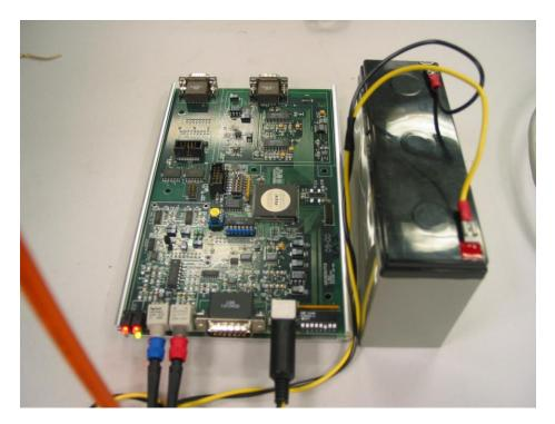
FIG 2A. Charge amplifier four channel electrometer. It is placed into a box measuring 9" x 5.5" x 2.5". This is the ADCMOD2 version, at 13ID (photo by Mark Rivers). Battery power lowers the noise.
