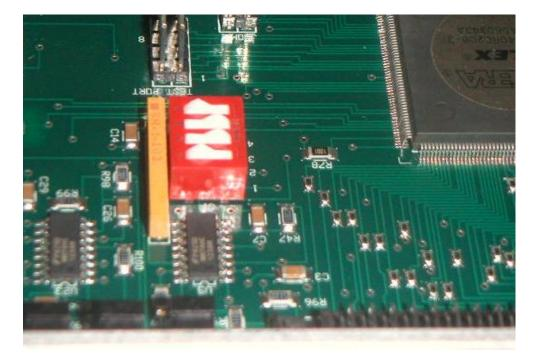
**6.4 JUMPERS.** Jumpers have no effect on my VME boards, but are necessary for other VME cards placed further to the right of mine in the VME crate. For initial tests, I recommend a mostly empty crate, so these are not issues. But as the crate fills up, they become important. The jumpers must be installed to pass the VME bus grants, and interrupt acknowledge to VME cards to the right of mine.
