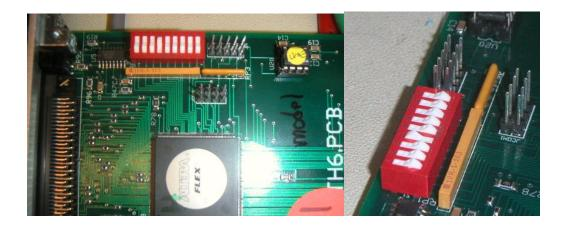
**6.3.4 PASSTH4,6 VSB side**. When the side of the switch closest to the VME side edge of the PCB is UP, then the switch is a logical low.
