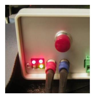
After step (4) above, the VME receiving continuous data via the orange fiber, to the bottom channel 0 of the FIBER2. The ADCMOD's top left light indicates data is flowing from it.
